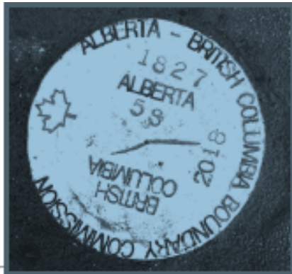
(Brass Cap monument in concrete base)
